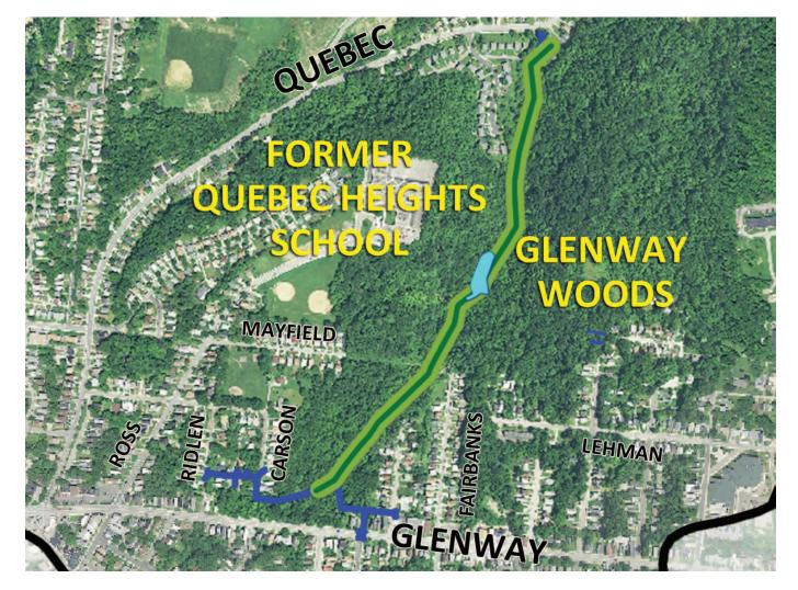
**Project Description:** Stormwater will be separated from a combined sewer that runs through Glenway Woods Park and will be redirected aboveground to a restored streambed. An existing low-lying area (see blue area) will be enhanced to slow and hold stormwater. New stormwater sewers will be installed along Ridlen, Wessels, Carson, and Drott avenues.
