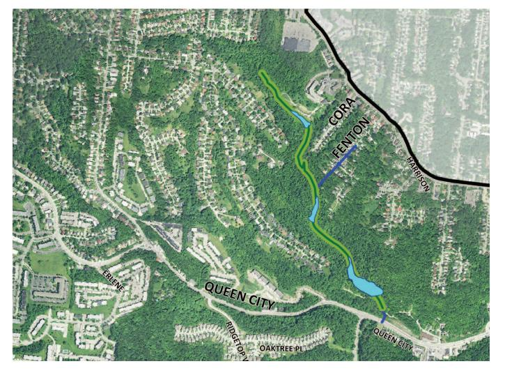
**Project Description:** Stormwater will be separated from a combined sewer that runs behind Judson Care Center and will be redirected aboveground to a restored streambed. Three low-lying areas (see blue areas) will be enhanced to slow and hold stormwater. New stormwater sewers will be installed along Fenton Avenue and at bottom of ravine.
