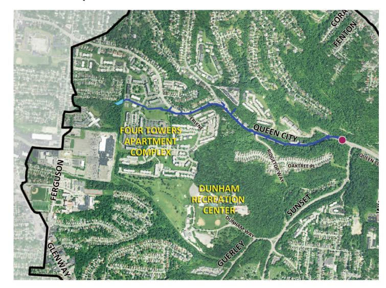
**Project Description:** Installation of approximately 6,000 linear feet of stormwater sewer and 1,500 feet of combined sewer along the northern side of Queen City Avenue from Sunset Avenue to an apartment complex off of East Tower Drive. An existing stormwater detention basin will be upgraded.
