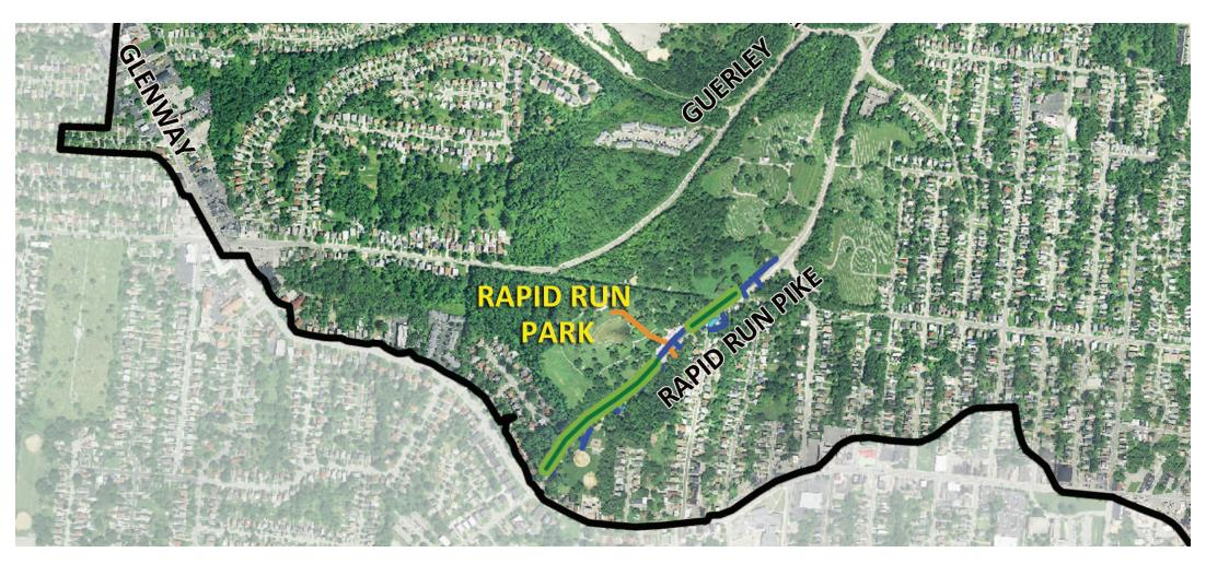
**Project Description:** About 1,600 linear feet of bioswale will be constructed on the park grounds parallel to Rapid Run Pike. The bioswale will carry stormwater runoff from the park, Rapid Run Pike and the hillsides/grounds on the south side of Rapid Run Pike, including the CRC playground and ballfield.
