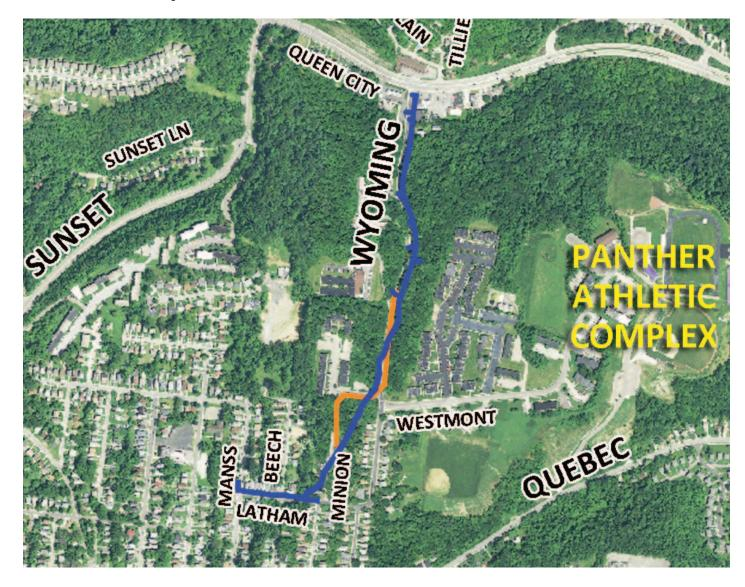
**Project Description:** About 3,100 linear feet of stormwater sewer will be installed along Wyoming Avenue and multiple side streets: Westmont Drive, Beech Avenue, Latham Avenue, Minion Avenue, and Manss Avenue.
