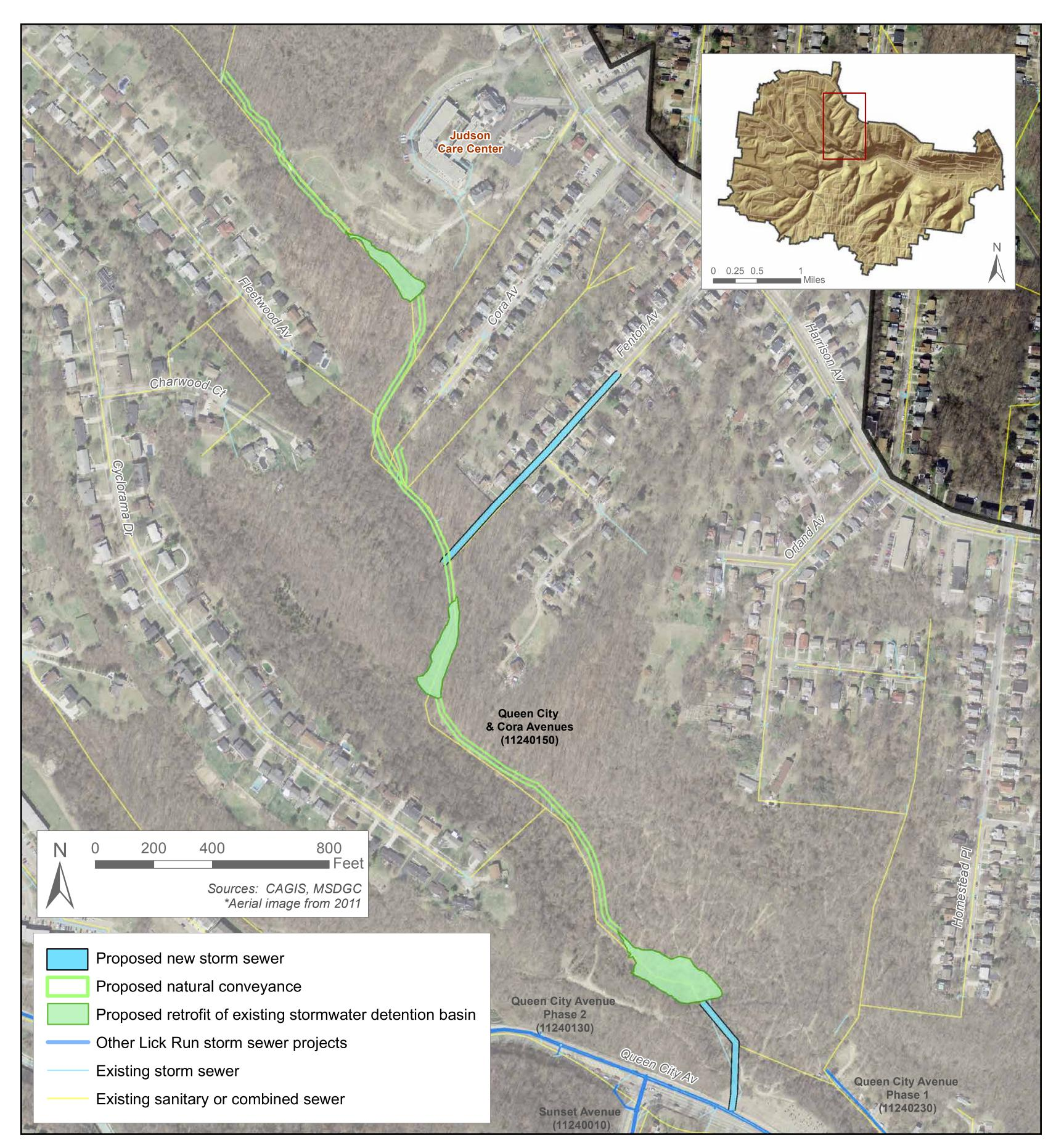
**Project Description:** Green infrastructure project in ravine behind Judson Care Center. Restoration of a stream that was enclosed in a combined sewer. Includes the retrofit of three existing stormwater detention basin and new storm sewer along Fenton Avenue and at bottom of the ravine. It will connect to storm sewers along Queen City Avenue.
