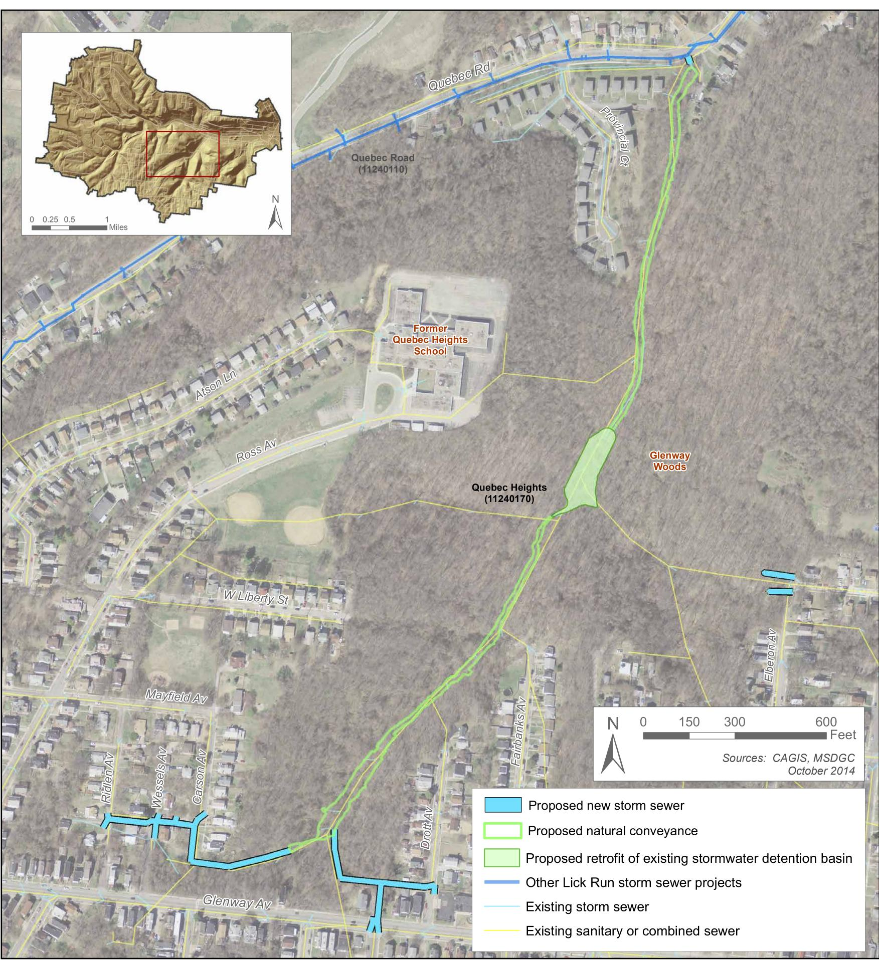
**Project Description:** Green infrastructure project in Glenway Woods. Restoration of a stream that was enclosed in a combined sewer. Includes the retrofit of one existing stormwater detention basin and new storm sewer across Glenway and along Ridlen, Wessels, Carson and Drott avenues. It will connect to storm sewers along Quebec Road.
