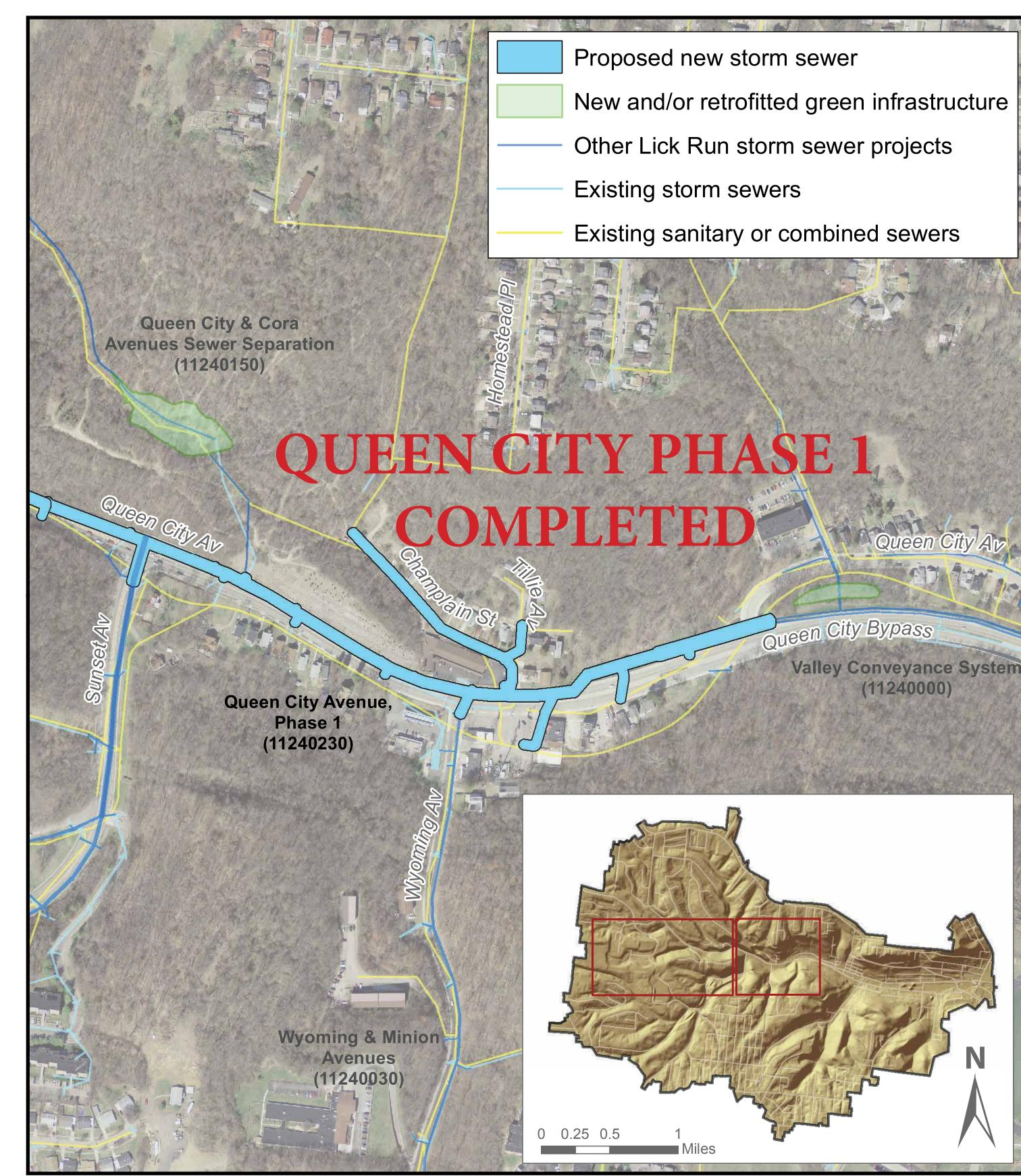
**Project Description:** About 6,000 linear feet of new storm sewer will be installed along Queen City Avenue between Sunset Avenue and an apartment complex off East Tower Drive. This project also includes the retrofit of one existing stormwater detention basin behind the apartment complex. This project will connect to storm sewers along Queen City Avenue.
