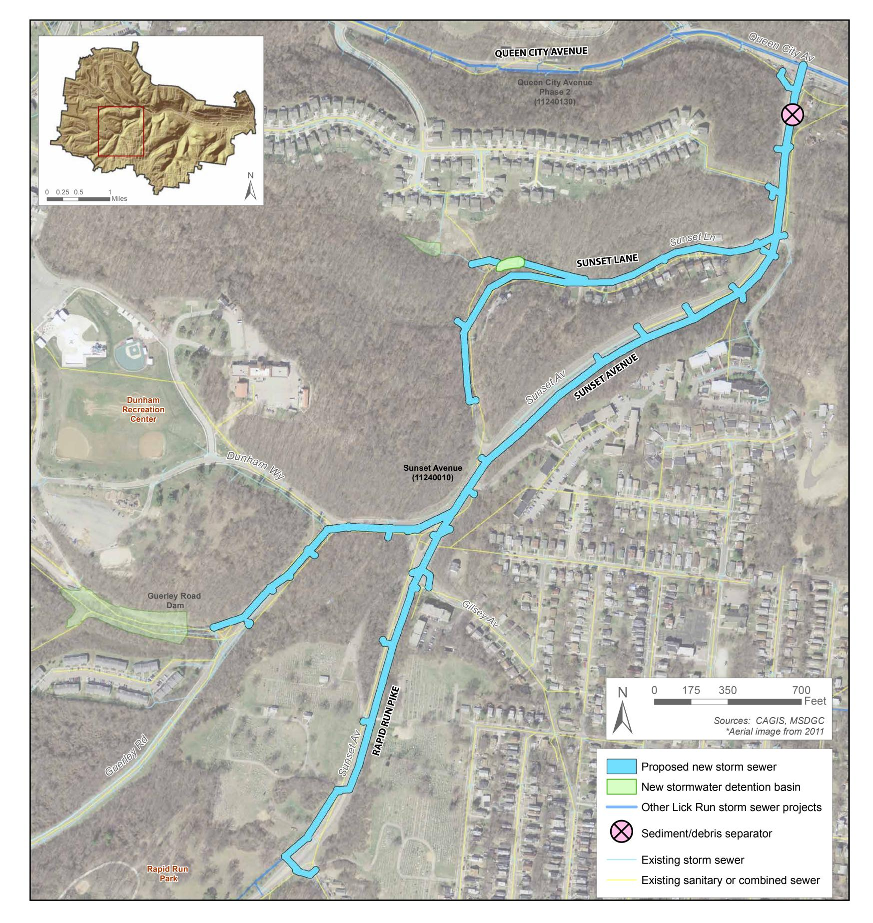
**Project Description:** About 10,000 linear feet of new storm sewer will be installed along Sunset Avenue/Rapid Run Pike, Sunset Lane and Guerley Road. A new stormwater detention basin will be constructed off Sunset Lane. An existing detention basin will also connect to the project. The sewers will connect to the Guerly Road detention dam and the Rapid Run Park bioswale and also to storm sewers along Queen City Avenue.
