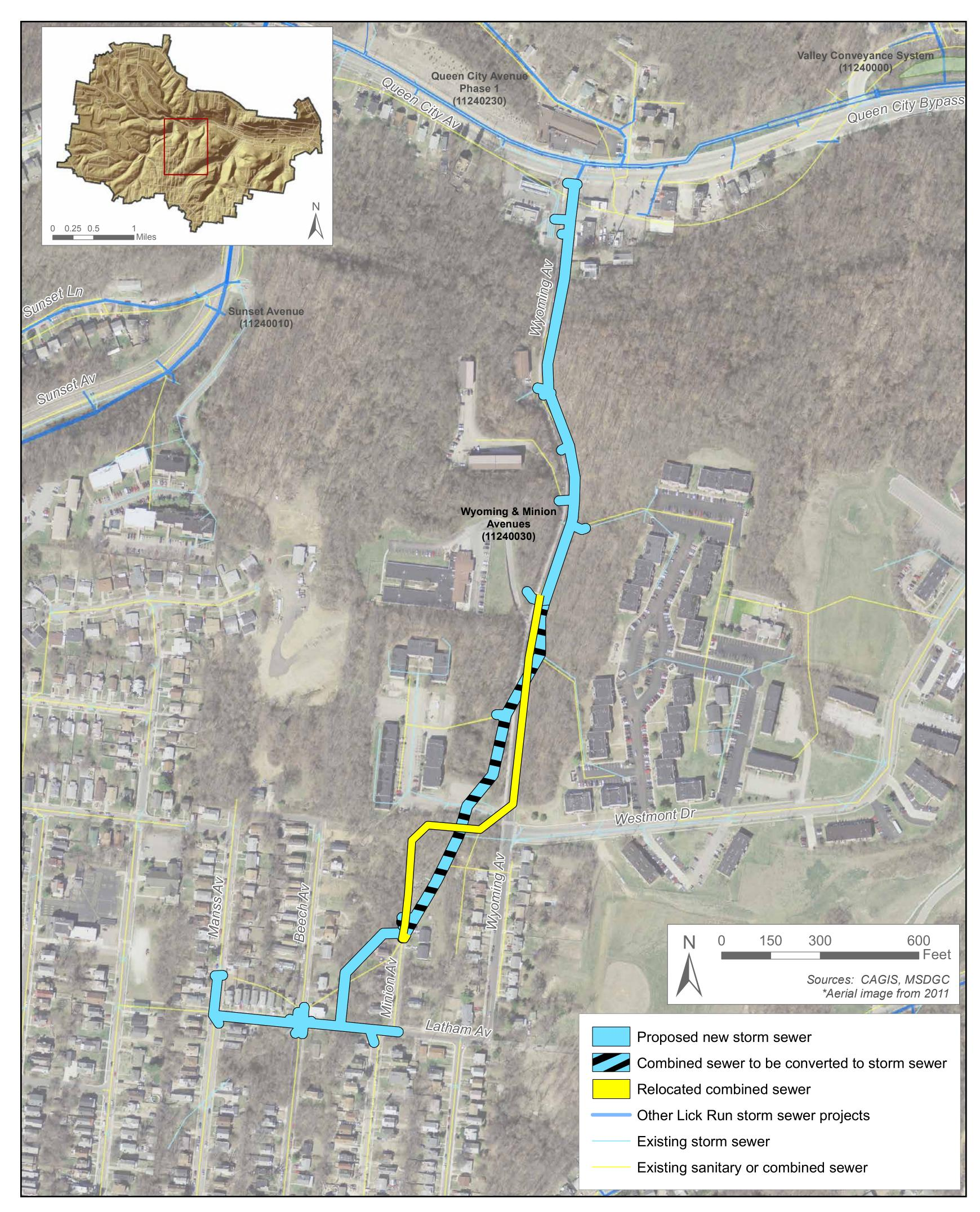
**Project Description:** About 3,100 linear feet of new storm sewer will be installed along Wyoming Avenue and multiple side streets: Westmont Drive and Beech, Latham, Minion and Manss avenues. It will connect to storm sewers along Queen City Avenue.
