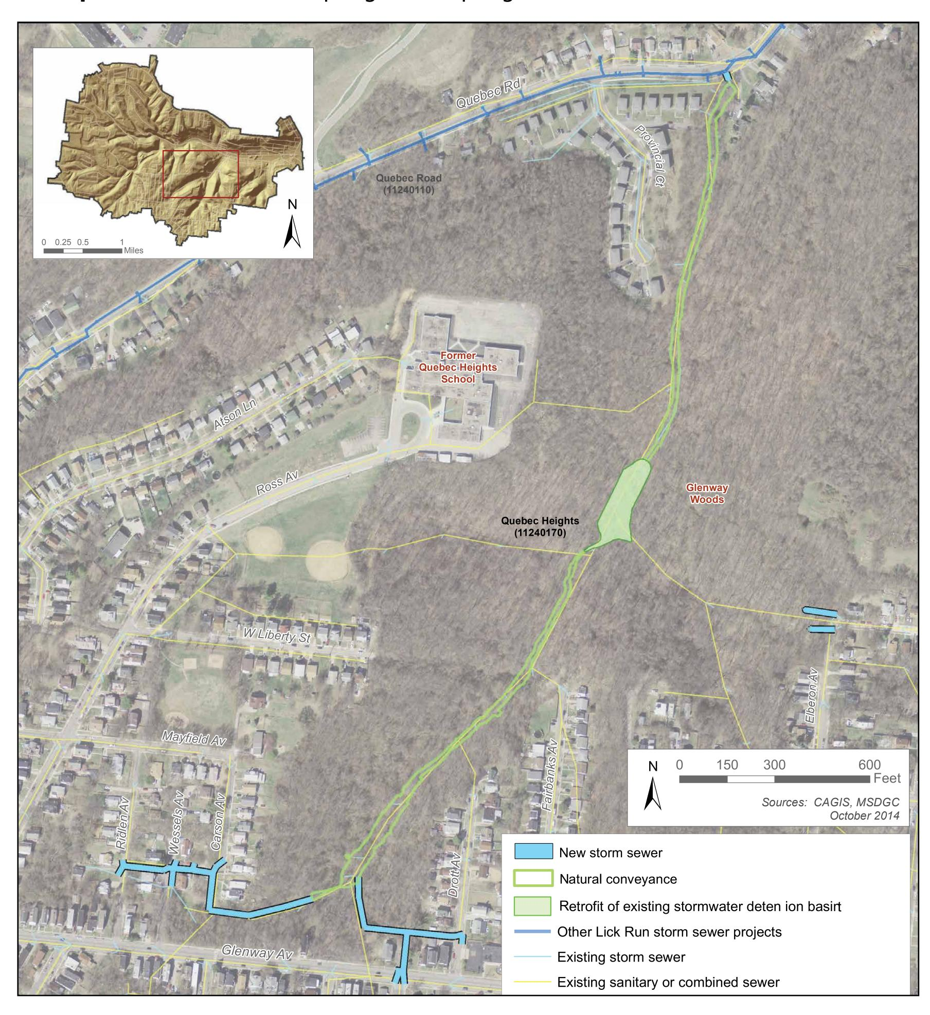
**Project Description:** Green infrastructure project in Glenway Woods. Restoration of a stream that was enclosed in a combined sewer. Includes the retrofit of one existing stormwater detention basin and new storm sewers across Glenway and along Ridlen, Wessels, Carson and Drott avenues. It will connect to storm sewers along Quebec Road.
