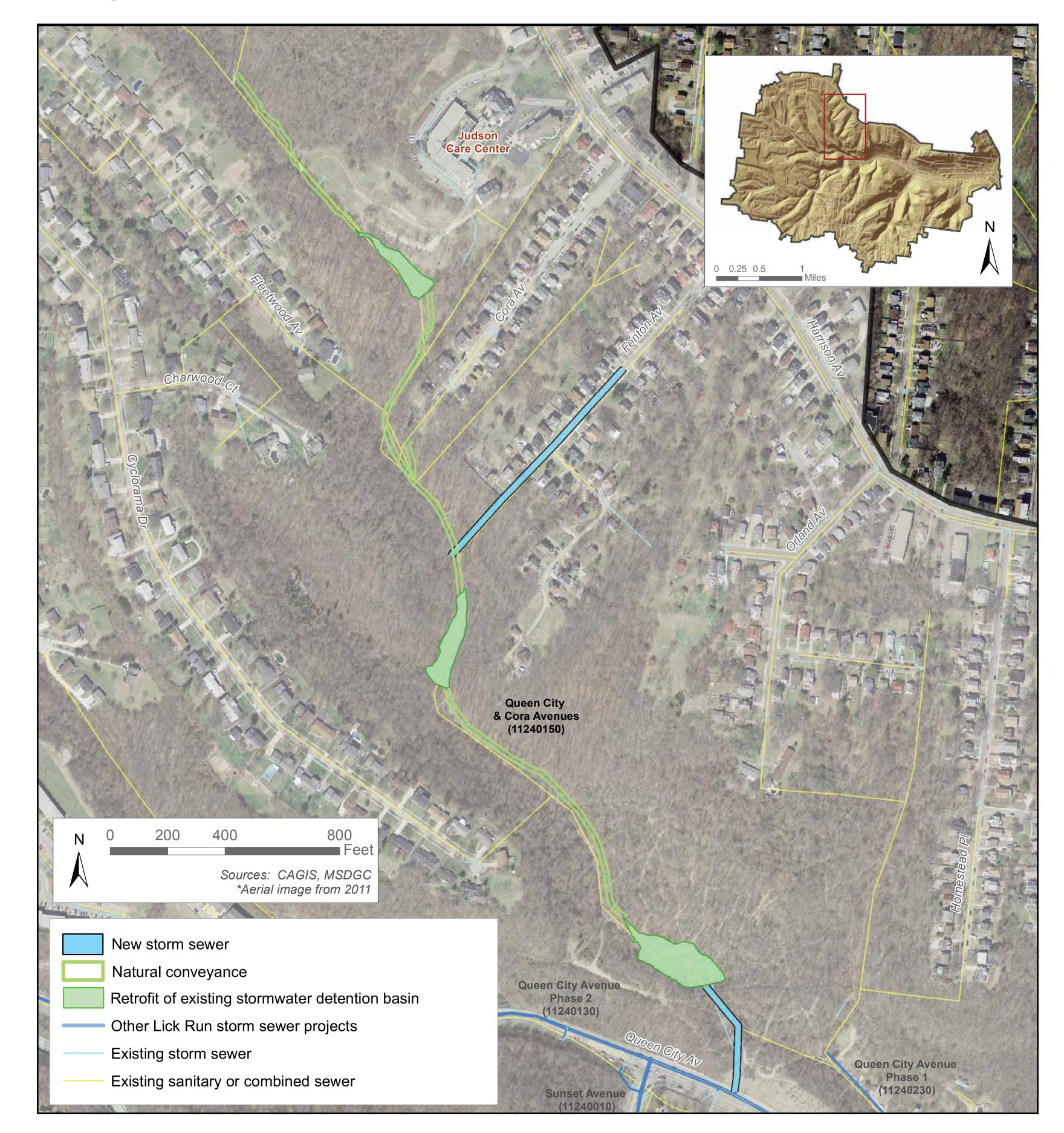
**Project Description:** Green infrastructure project in ravine behind Judson Care Center. Restoration of a stream that was enclosed in a combined sewer. Includes the retrofit of three existing stormwater detention basin and new storm sewers along Fenton Avenue and at bottom of the ravine. It will connect to storm sewers along Queen City Avenue.
